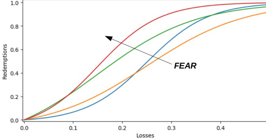
Figure 1: This shows different examples of the redemption function, each with a different fear. The arrow intuitively shows how more fear in the market affects the shape of the redemption function.
