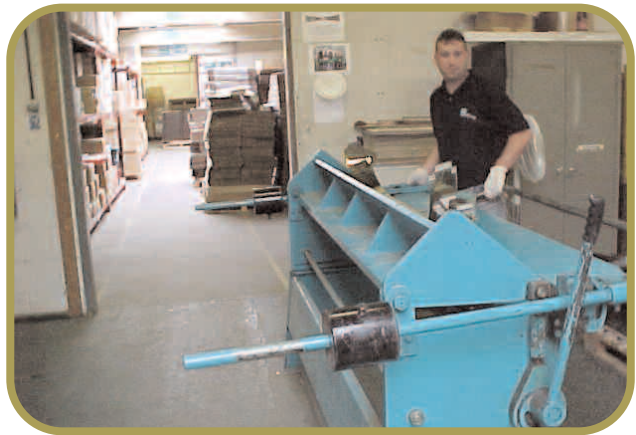
Guillotine obstructing aisle when in operation
